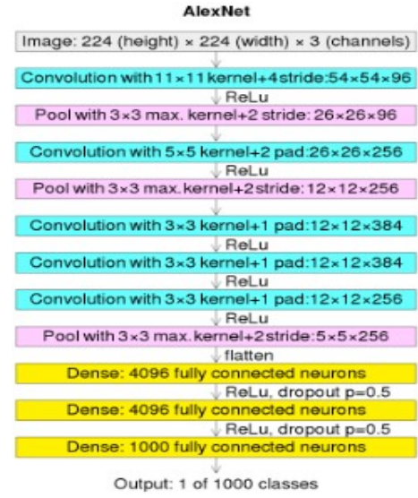
Figure 9: The 8 layers of AlexNet (See [31])
